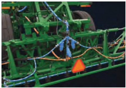
Pressure Recirculation & Product Reclaim
