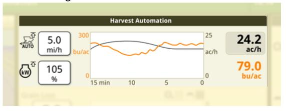
The limiting factor for Ground Speed Automation is shown to the right of the GSA icon when Automation is in control (blue text).
